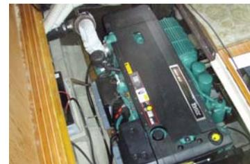
SF38 repowered by Volvo Penta D6-435/HS80AE(1.96:1)x2 Twin 3箇所操作仕様+Low Speedオプション付き
